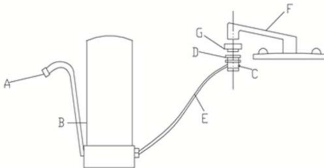
A. spout; B. housing; C. button; D. diverter valve; E. hose; F. faucet; G. adapter
